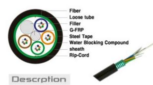
loose tube style, optical fiber cable with non-metallic central strength member of G-FRP and peripheral strength members with moisture barrier inner sheath. Cable protected by black PE over sheath, suitable for duct or aerial application. Tubes contain optical single-mode or multimode fibers.
