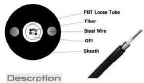
Non armored optic cable, single-mode/multimode fibres are positioned in the loose tube, which is made of high modulus plastic materials and filled with filling compound. jelly filled and fiber contained central loose tube, two parallel steel wires. Suitable for duct or aerial application. Tubes contain optical fibers colour coded.
